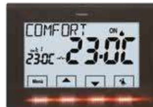
Above 21,1 °C the keys light up in red indicating consumption over needs
