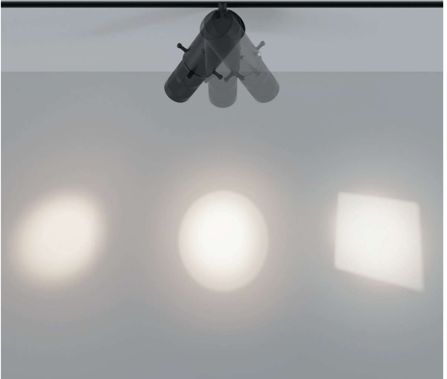
A telescopic lens mechanism allows you to adjust the projection angle from 20° to 35°.
